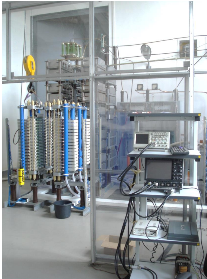
IGBT valve testing lab
